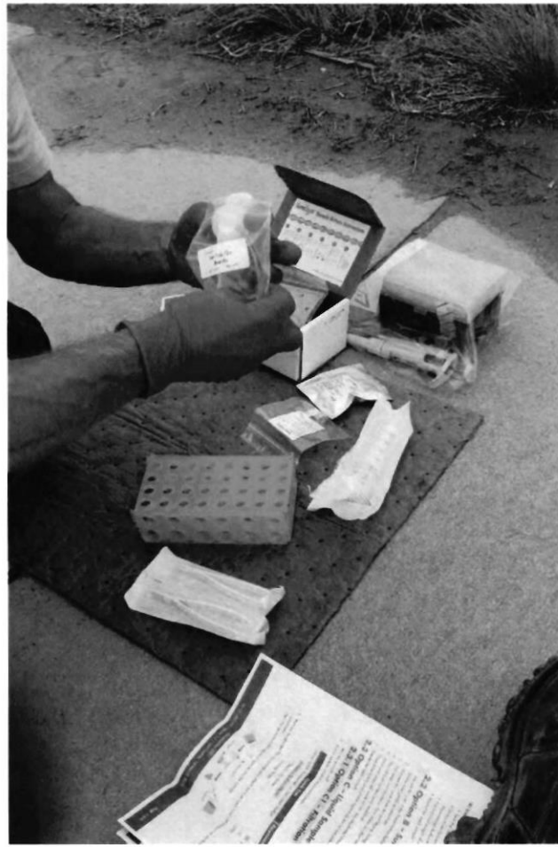
Photograph 2. DNA trace kit; to be filtered and preserved in the field.
